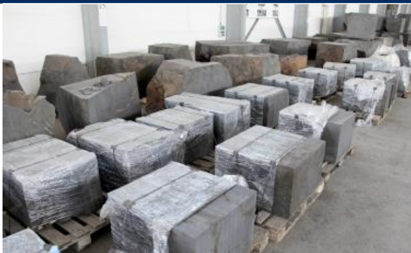
Figure 2: Blocks of mined ore cut into 50kg electrodes for feeding exfoliation cells
