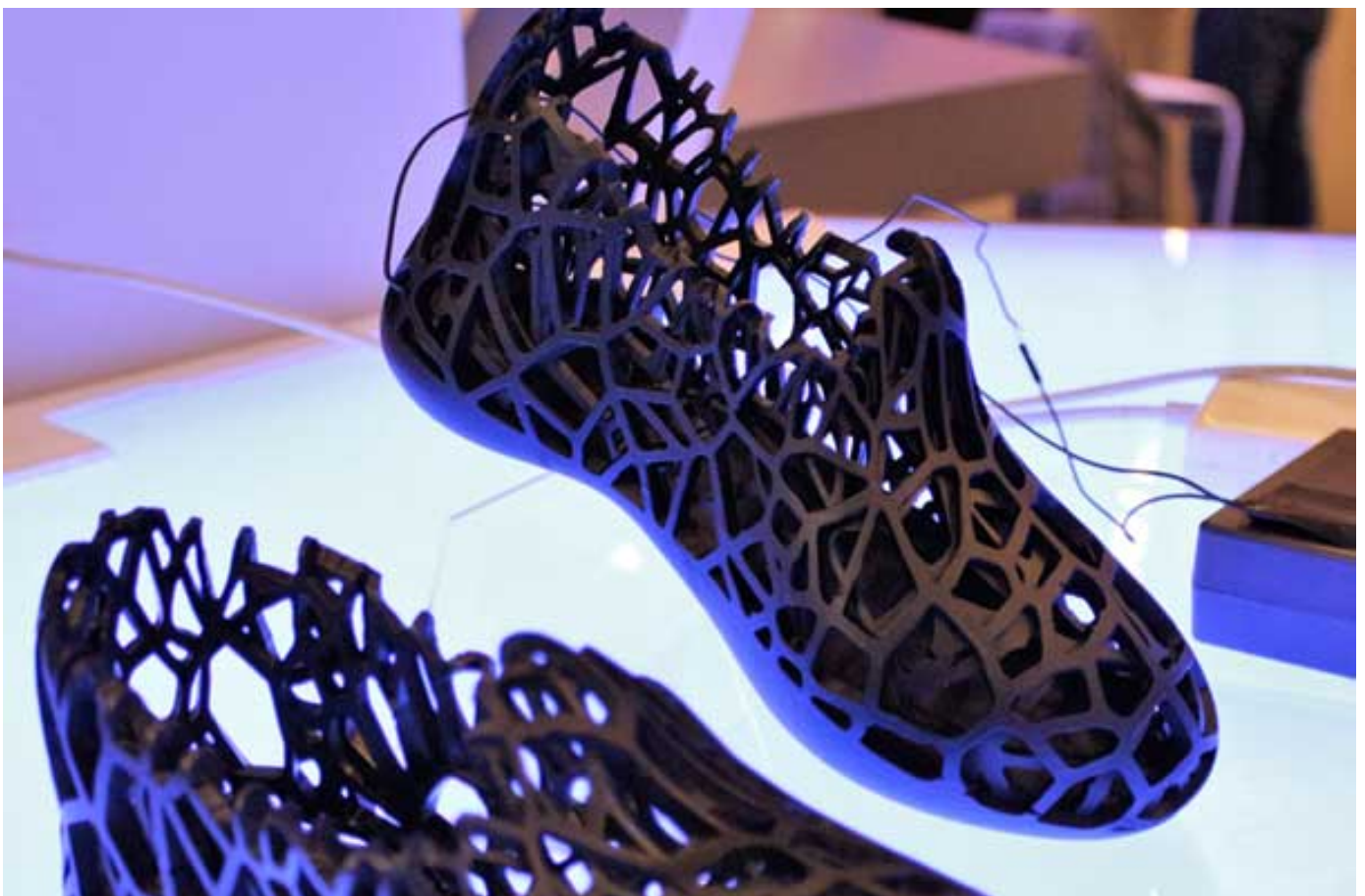
3D-printed pressure sensor shoe
